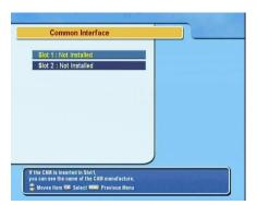
To view the information about the module and subscription card inserted into the digital receiver, select the Common Interface menu. You should see a screen like the left figure.
